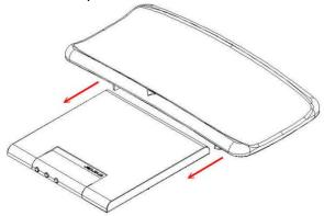
2. Turn device upside down. Secure tray to device by turning knob on each side of tray. (turn clockwise to tighten, turn counter-clockwise to loosen)
