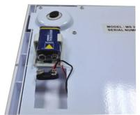
5. Place battery into housing. Close cover and turn scale right-side up. Power on device to test if batteries are installed correctly.
