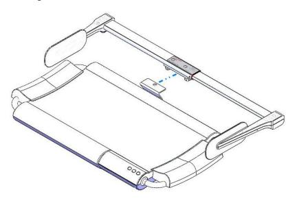
3. To detach height measure, find the latch located at the rear of the attachment. Press down on the buckle, and gently remove the attachment from bracket.
